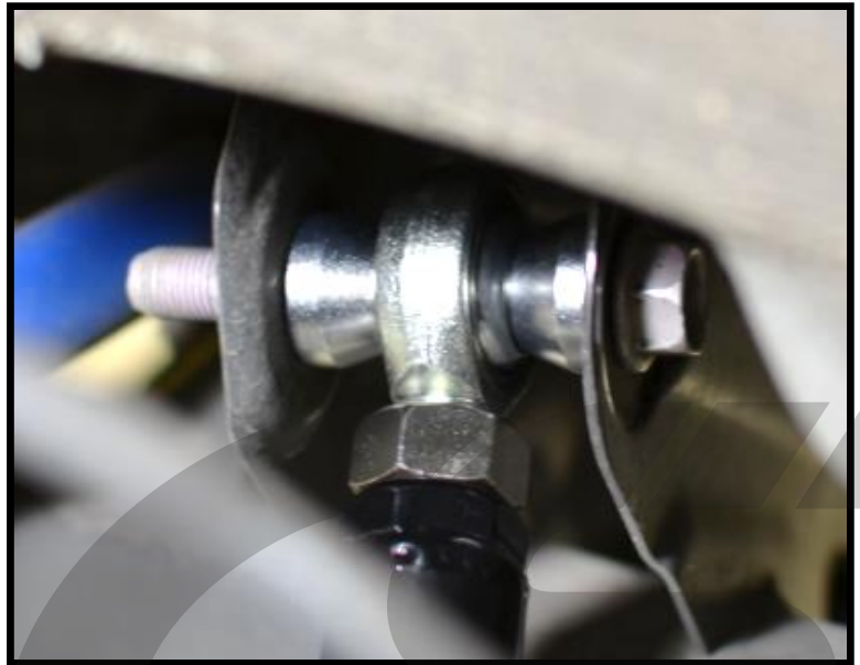
Figure 3b: Correct Alignment
