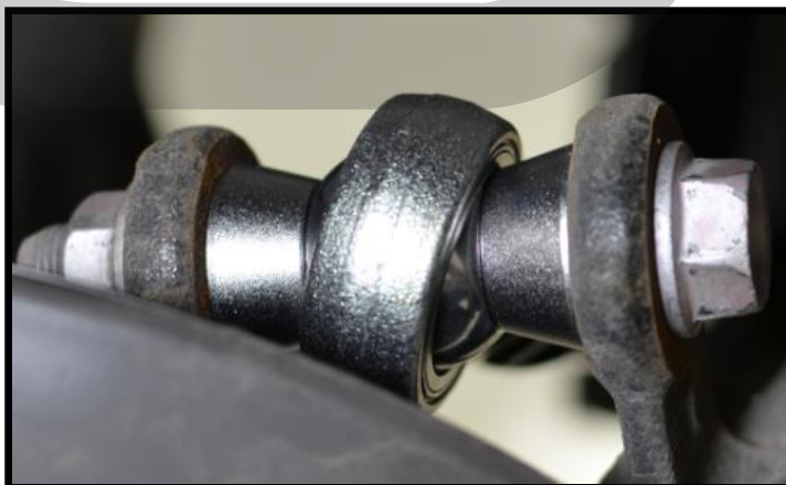
Figure 3d: Incorrect Alignment
