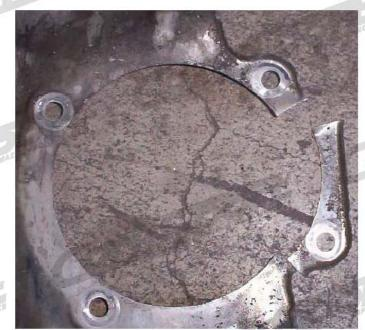
Step 9: Grind the points on the hub so that the new brake rotor slides over the hub and fits snugly. This will require removing small amounts at a time and test fitting until the rotor fits.
