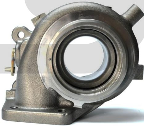
Figure 2: Turbine housing cartridge side (left) and outlet side assembled (right).
