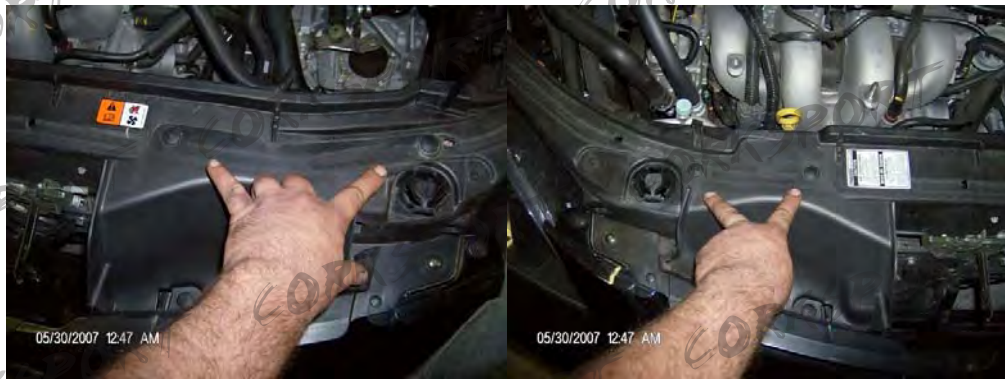
Step 26: Remove two Phillips head screw type clips from corners of bumper grill.
