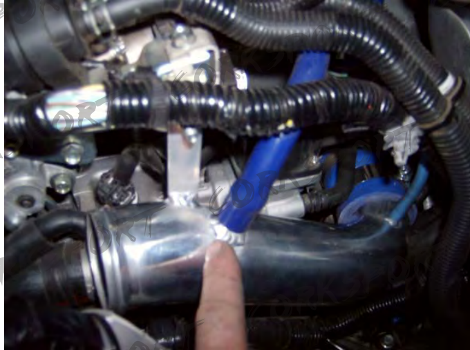
Step 25: Remove the four Phillips head screw type clips from inlet ducts to core support.
