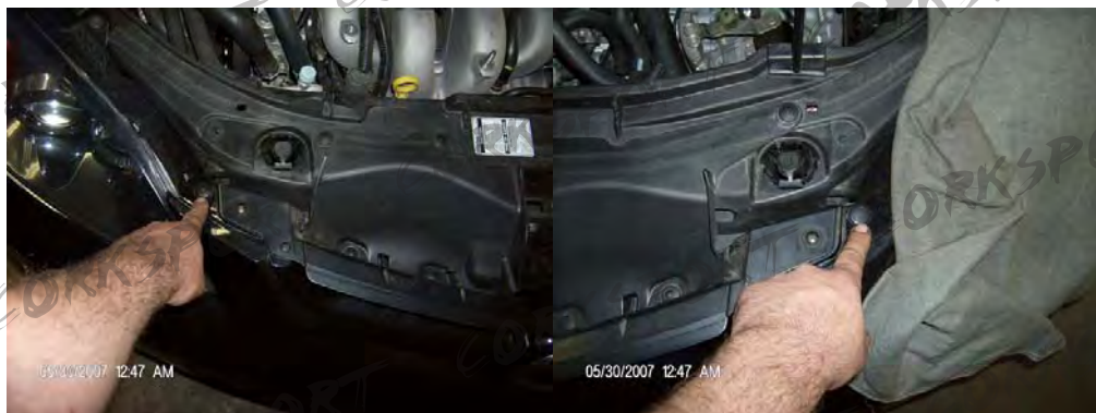
Step 26: Remove two Phillips head screw type clips from corners of bumper grill.
