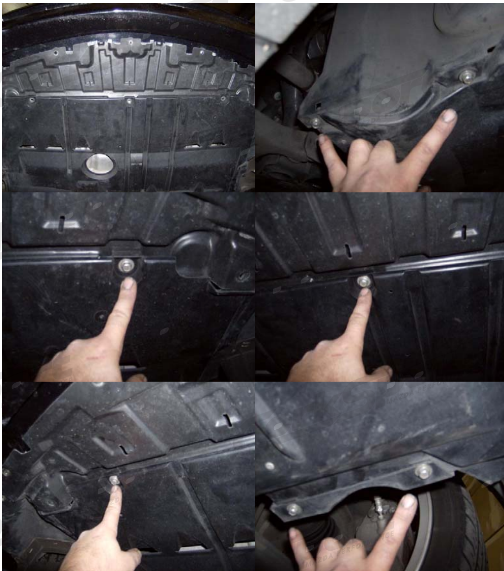
Step 18: Reinstall main under tray with original seven (7) 10mm head bolts.
