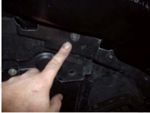
Step 18: Reinstall main under tray with original seven (7) 10mm head bolts.
