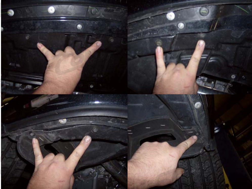
Step 6: Remove seven (7) 10mm head bolts from under tray and remove under tray.
