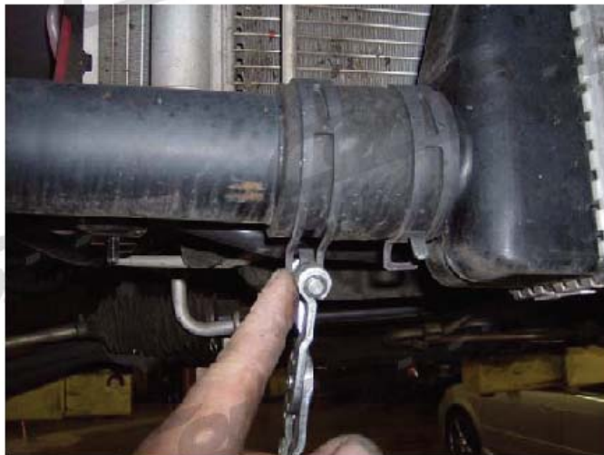
Step 37: Using pliers squeeze the hose clamp on the intercooler and remove the intercooler pipe from the Miata
