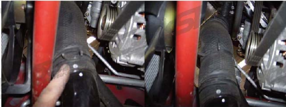
Step 37: Using pliers squeeze the hose clamp on the intercooler and remove the intercooler pipe from the Miata
