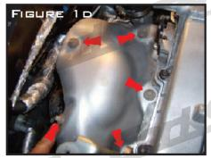
INFILTRATE ALL OF THE THREADS. MAKE SURE NOT TO TWIST THE WIRING HARNESS UP WHEN REMOVING THE SENSOR. YOU CAN DISCONNECT IT AT THE PLUG IF NECESSARY, BUT THERE IS PLENTY OF SLACK TO REMOVE THE SENSOR AND AVOID TWISTING THE CABLE.
