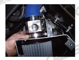
Step 8: Install air box lid with the 5 M8 Socket Head Cap Screws around the perimeter of the box using your 6mm head Allen wrench. These should just be hand tight. You may need to compress the foam sealing tape slightly with the lid in order to get the screws started.
