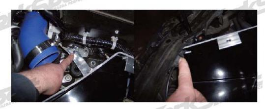
Step 5: Reinstall factory 10mm head nut onto the bracket and hand tighten.
