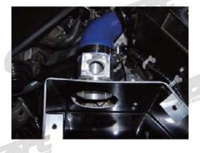
Step 7: Install filter through airbox and onto MAF housing. Unbolt second T-Bolt clamp entirely and attach around air filter. Tighten clamp using 10mm deep socket. Tighten the all three bracket fasteners (between the box & bracket as well as between the bracket & car) to ~8 ft lb of torque.
