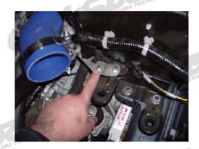
Step 4: Remove lid from air box. Install air box so that bracket goes onto stud pictured and slot in front side of air box fits into space in core support. This installation is fairly tight and may require that you loosen the fasteners between the bracket and the box.
