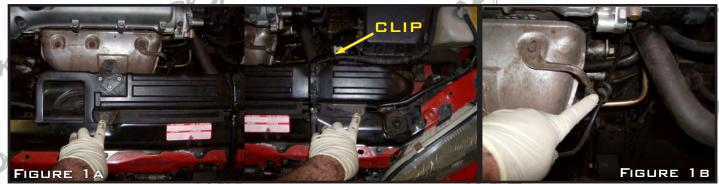
B. DETACH THE Q2 SENSOR WIRE (SHOWN IN **FIGURE 1B**) THAT IS ATTACHED TO THE COILED CLIP ON THE HEAT SHIELD BY UNWINDING IT OUT OF THE COIL.
