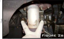
C. USING A 14MM SOCKET AND 14MM WRENCH, REMOVE TWO 14MM DOWNPIPE NUTS/BOLTS THAT
